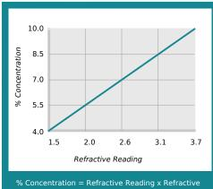
6 Concentration = Refractive Reading x Refractive Factor Coolant Refractometer Factor % Brix = 2.7
