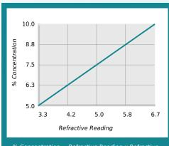
% Concentration = Refractive Reading x Refractive Factor Coolant Refractometer Factor % Brix = 1.5
