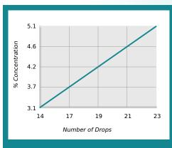
% Concentration = No. of Drops x Titration Factor Titration Factor = 0.22
