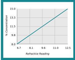
% Concentration = Refractive Reading x Refractive Factor Coolant Refractometer Factor % Brix = 1.2
