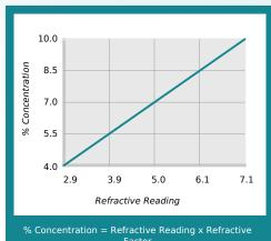
Coolant Refractometer Factor % Brix = 1.4
