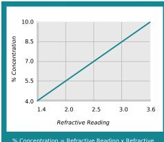
% Concentration = Refractive Reading x Refractive Factor Coolant Refractometer Factor % Brix = 2.8
