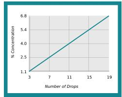
% Concentration = No. of Drops x Titration Factor Titration Factor = 0.36
