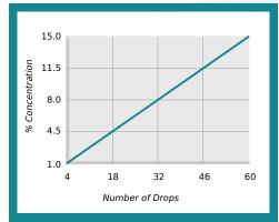
% Concentration = No. of Drops x Titration Factor Titration Factor = 0.25
