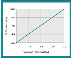
% Concentration = Refractive Reading x Refractive Factor Coolant Refractometer Factor % Brix = 3.4
