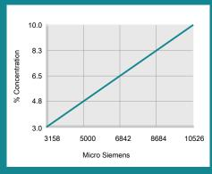
% Concentration = Conductivity in Micro Siemens x Factor Conductivity Factor = 0.00095
