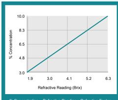
% Concentration = Refractive Reading x Refractive Factor Coolant Refractometer Factor % Brix = 1.6
