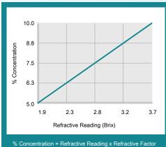
6 Concentration = Refractive Reading x Refractive Factor Coolant Refractometer Factor % Brix = 2.7
