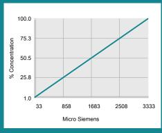
% Concentration = Conductivity in Micro Siemens x Factor Conductivity Factor = 0.03000
