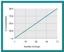
% Concentration = No. of Drops x Titration Factor Titration Factor = 1.40
