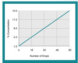
% Concentration = No. of Drops x Titration Factor Titration Factor = 0.25
