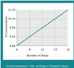
% Concentration = No. of Drops x Titration Factor Titration Factor = 0.78
