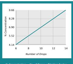
6 Concentration = No. of Drops x Titration Factor Titration Factor = 0.69
