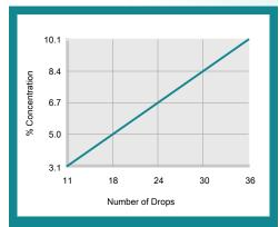
% Concentration = No. of Drops x Titration Factor Titration Factor = 0.28
