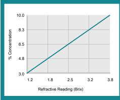
% Concentration = Refractive Reading x Refractive Factor Coolant Refractometer Factor % Brix = 2.6
