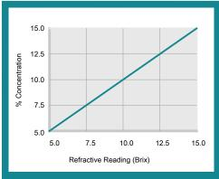
% Concentration = Refractive Reading x Refractive Factor Coolant Refractometer Factor % Brix = 1.0
