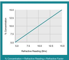
6 Concentration = Refractive Reading x Refractive Factor Coolant Refractometer Factor % Brix = 1.0
