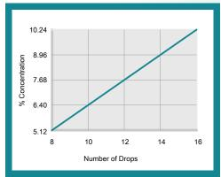
% Concentration = No. of Drops x Titration Factor Titration Factor = 0.64
