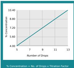
% Concentration = No. of Drops x Titration Factor Titration Factor = 0.80
