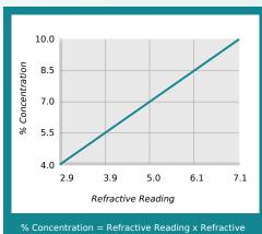
% Concentration = Refractive Reading x Refractive Factor Coolant Refractometer Factor % Brix = 1.4
